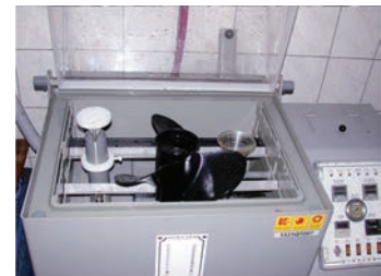
Salt Water Spray Testing
